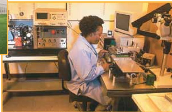
▶ Autotyping center packages chips into waffle packs
