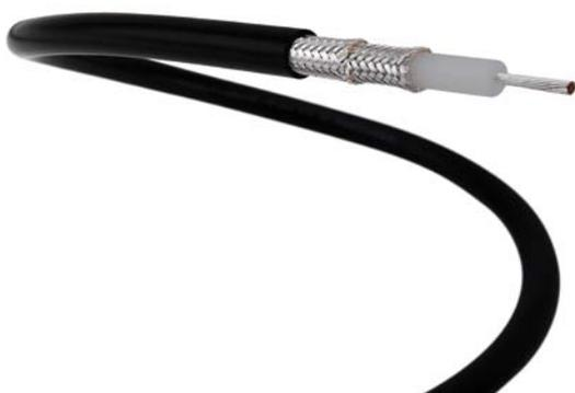
HUBER+SUHNER cross-linking technology in combination with low loss dielectrics makes this product portfolio outstanding. Cross-linking allows the maximum application temperature of polyethylene to be increased from +80 to +105 °C. This extended range covers most applications. It allows operation in a higher power range and connectors with soldered inner conductors can be easily applied.
